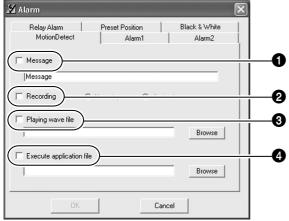
(Setting of **1** and **2** are disabled when in the Relay Alarm mode.)
